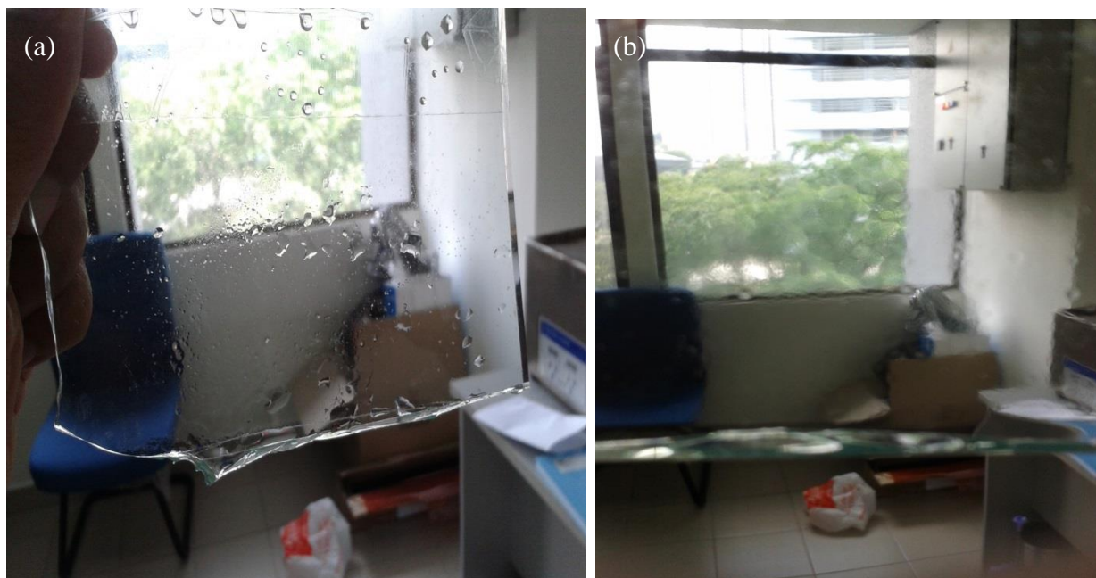
Fig 6: The Formation Of Dirt Layer On (A) Bare Glass And (B) Coating Glasses
