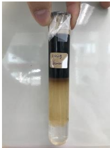
Figure 5: Micro-emulsion of 0.1wt% of Gemini Surfactant.
