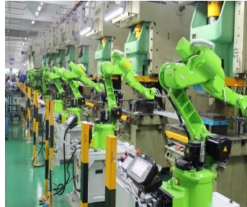
Figure 3 : Articulated Robots Installation Along With Stamping Machines Line
