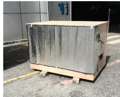
Fig. 7 Test room insulated with PASB
