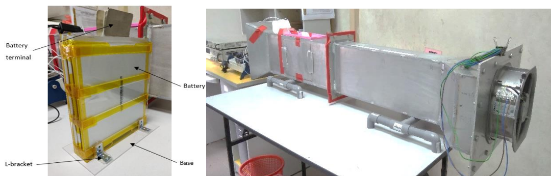
Fig. 2. Completed battery module and air tunnel
