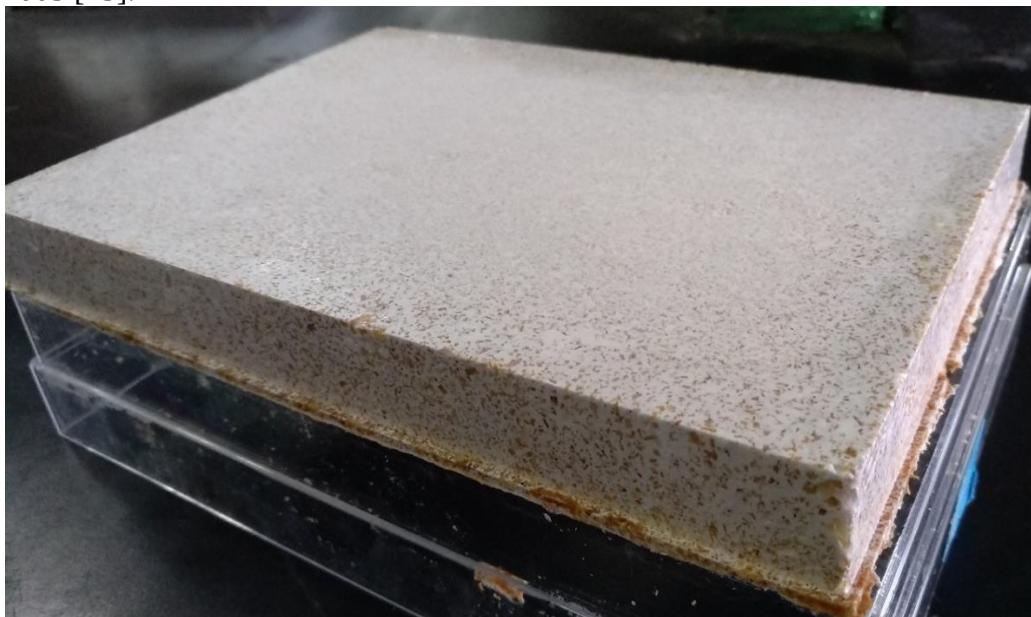
Fig. 2 Bio-composite from RWS inoculated with mycelium before hot press.
