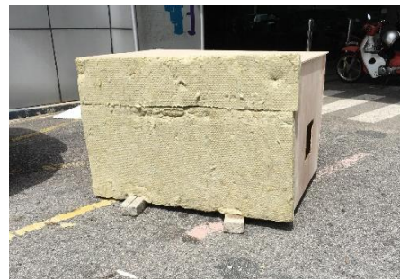
Fig. 9 Test room insulated with Rockwool
