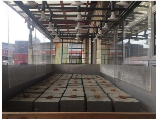
Figure 5 : Integrated GSI Arrangement Inside The Rainfall Simulator
