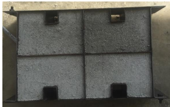
Figure 4 : Steel Mould Used To Case Integrated GSI
