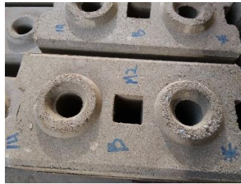
Figure 7. Rough surface of ICB18.
