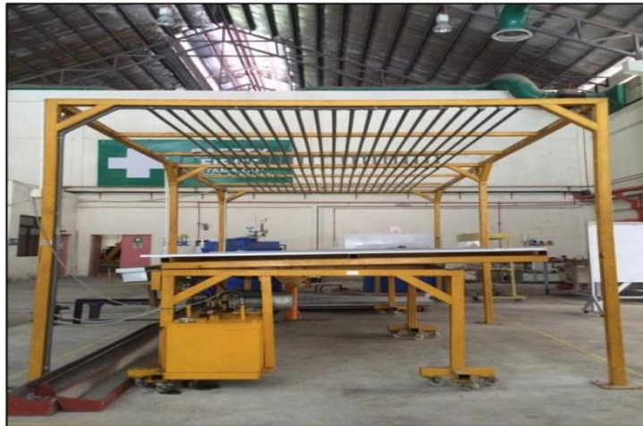
Figure 4: Testing under a rainfall simulator
