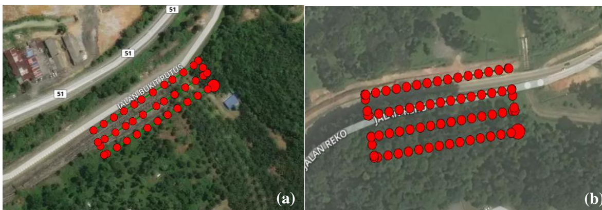
Figure 1. Images of slope with grid mission flight using Pix4Dcapture at location (a) Jalan Kuala Pilah and (b) Jalan Bangi
