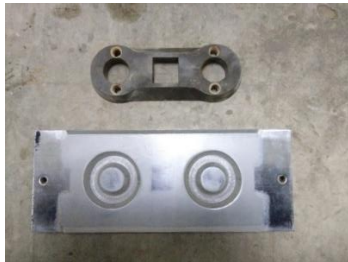
Figure 6. Metal plate used for compressive strength test.
