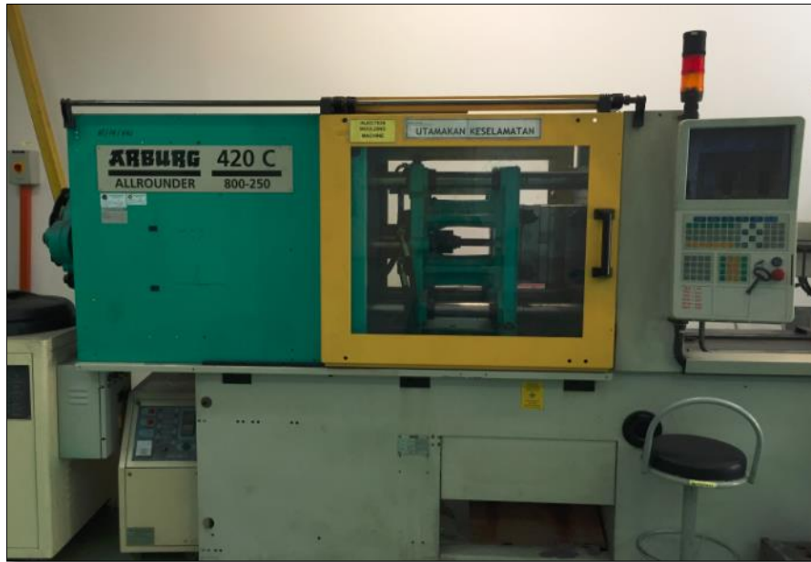
Figure 3.3: Injection Molding Machine Used In The Experimental Work.
