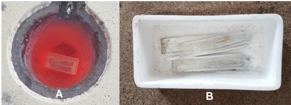
Figure 6: (A) Specimen Sample in Ceramic Cubicle placed in the Crucible Furnace, (B) Remains of Fibre after Burnout Test
