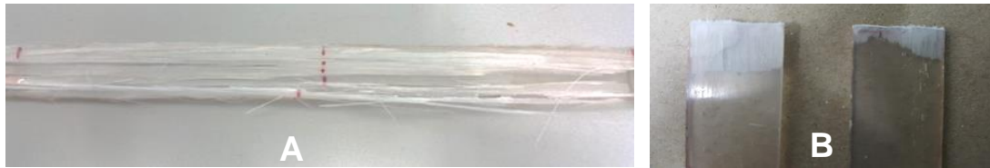
Figure 2: (A) Fractured Test Specimen from Preliminary Tensile Test, (B) Fractured Test Specimen After an Incision Was Introduced.
