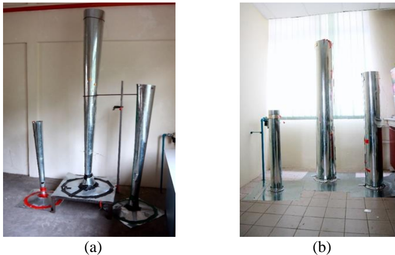
Figure 11:(A) Divergent Chimneys (B) Cylindrical Chimneys
