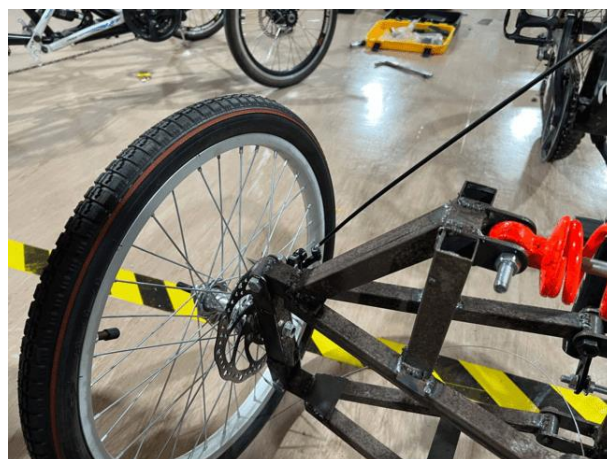
Figure 15: The Cable Brake Has Been Attached.
