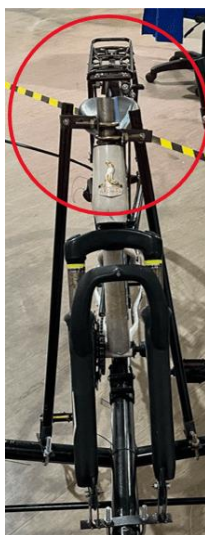
Figure 4: The Center Bar Which Will Be Removed.
