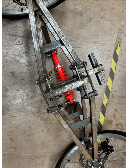
Figure 11: Before Sanding and Spray Paint Process Is Done.
