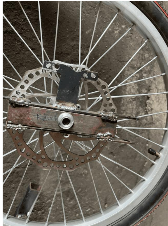
Figure 8: The Bracket Has Been Mounted.
