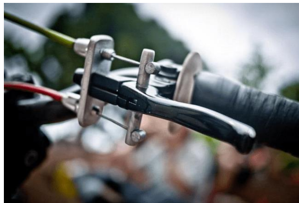
Figure 1: The Single Lever for The Double-Disc Brake System
