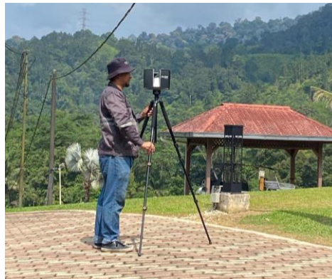
Figure 4: Terrestrial laser scanning activities using the FARO Focus M70 during data acquisition at the case study site
