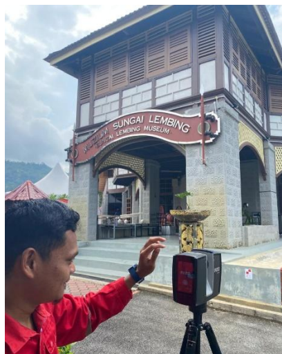
Figure 1: Muzium Sungai Lembing, Pahang, Malaysia: exterior and interior views of the heritage building selected as the case study for the Scan-to-HBIM implementation.
